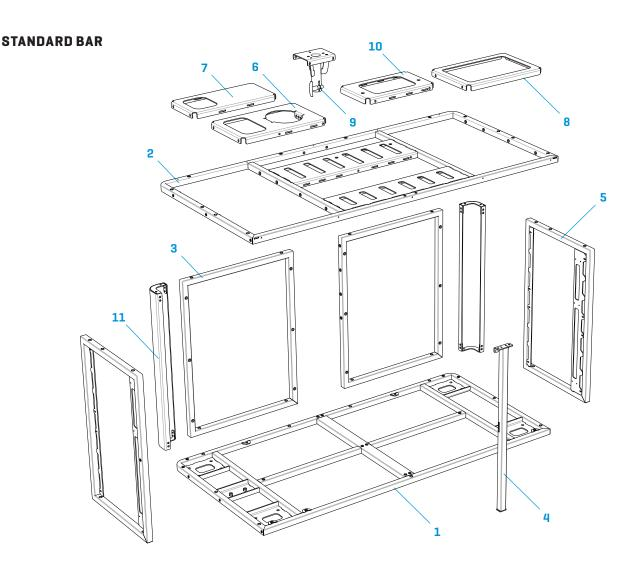
At the heart of the POP-UP BAR is the superstrong steel frame consisting of precision laser-cut and TIG-welded modules that are bolted together.
